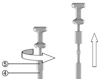
2. Unscrew the suction tip ③ and pull the piston ⑥ out of the tube.
